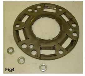
**6.** The new billet basket assembly is screwed together instead of riveting; you will need to drill out the spacers (fig 5) & the spring retainer (fig 6) that fits on to the new basket to a 10mm hole.
