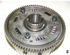
10. Torque the bolts up to 38lb/ft using a bar as shown.
