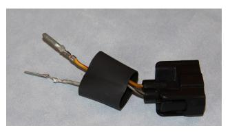
5. All the connectors have two wires, the 12v is the wire which is the same colour on all connectors, normally yellow with a red trace. Insert the terminals into the connector in the position shown below, ensuring that the terminals lock in.
