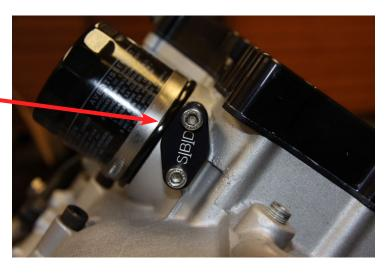
Alternatively, the outlet fitting can be moved to the bottom of the pump, the fitting may need to be machined in order to reduce the height of the fitting, this should provide sufficient clearance for the oil hose to run under the engine.
