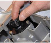
Using a straight edge across the underside of the pick up pipe as shown, you need to measure a gap on both sides of approximately 0.5mm. Due to the springy design of the o-rings, this will allow some accomodation if this dimension is greater than specified, but if the dimension is less than 0.5mm when gentle pressure is applied, to the oil pick up pipe, then add additional o-ring (shown below) supplied and recheck.
