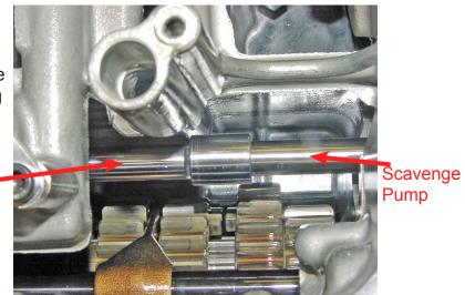
Fit a new Genuine Suzuki pick-up pipe O-ring (available from your Suzuki dealer), use a suitable grease to hold it in place during assembly.
