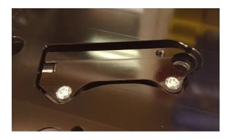
Addtional screw hole is only to aid installation & removal of the oil pressure relief valve holder.
