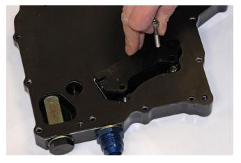
Apply a small amount of Loctite 243 retainer to bolts. Tighten the M6 x 16 bolt.
