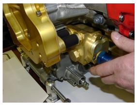
19 Secure the pump using the relevant bolts. Apply Loctite 243 to the flange retaining bolts and tighten
