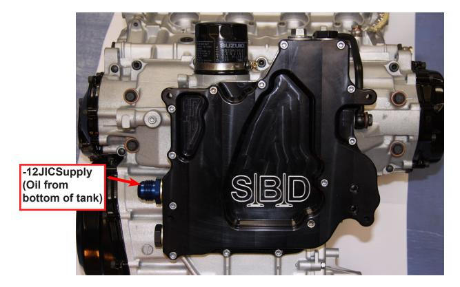
If required - Oil Cooler to be fitted on return line (scavenge) to tank
