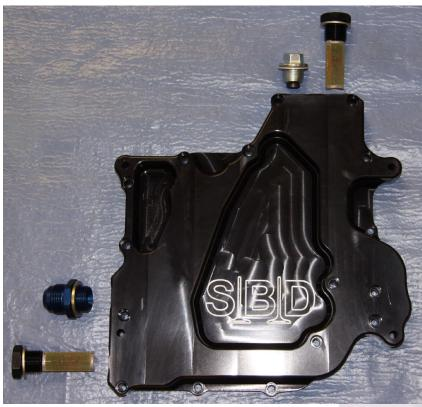
Insert the filters, coupling and blank
