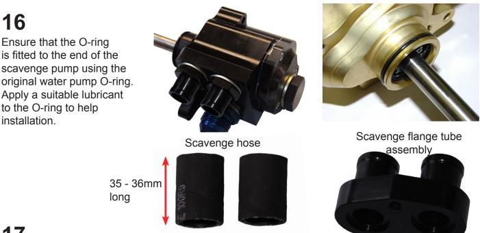
Because the scavenge pump (picture 17a) sits at a slight angle, to allow correct alignment the scavenge flange tube assembly is correspondingly machined to ensure correct alignment. To ensure you fit the assembly correctly, the tubes should tilt backwards as shown in 17b (17b also has scavenge joining hoses fitted). Once you have confirmed the correct direction, use a small amount of lubricant on to the inside of the hoses and press assembly together as shown in 17a.
