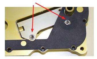
When fitting the sump ensure that the new relief valve connecting tube slides into position with a slight resistance, using the supplied bolts.
