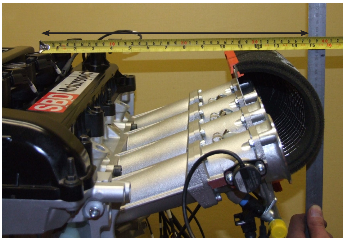
Centre of engine to outside edge of air filter - 378mm
