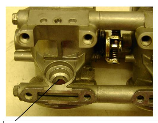
Modify the lower diameter for injector tip INJ-690P - 10.60mm INJ-330P & INJ-480P - 11.50mm
