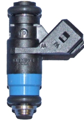
INJ-690P High flow injector, blue 690cc, 12.5 Ohms
