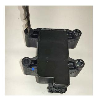
2. Drill out the two holes with the raised shoulder using an 8mm drill and just cut off the remaining raised shoulder with a Stanley knife so it is flat.
