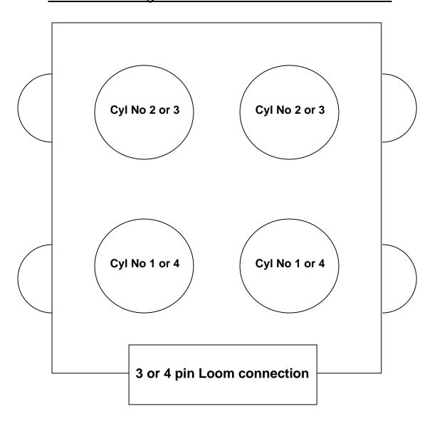
These coil packs, when used with the MBE ECU, use a wasted spark system. Both cylinders spark at the same time. That is why you can install 1 & 4 on either post & the same for 2 & 3.
