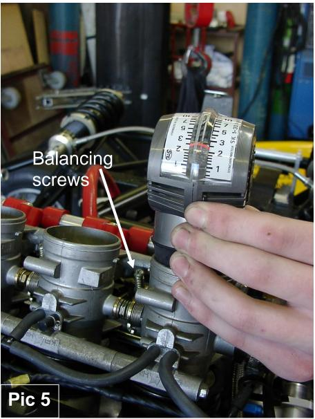
4. Once you have got the engine running, you can then balance the butterflies by using the screws in between the bodies as shown above
