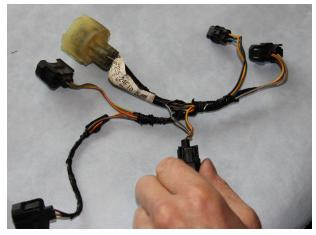
2. Cut each connector from the harness leaving 45mm of wire to allow the new connector to be fitted.
