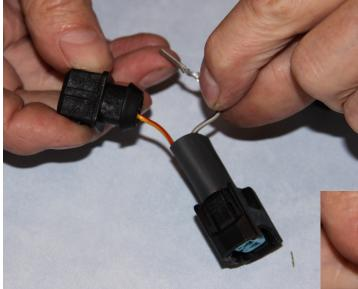
5. All the connectors have two wires, the 12v is the wire which is the same colour on all connectors, normally yellow with a red trace. Insert the terminals into the connector in the position shown below, ensuring that the terminals lock in.
