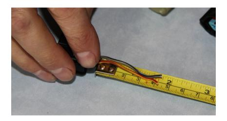
3. Strip approx 5mm of the covering insulation to expose bare wire. Crimp on the pins.
