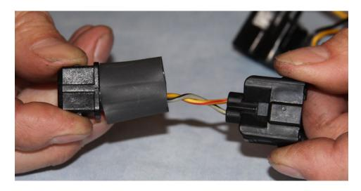
7. Move heat shrink in place and apply heat to shrink.
