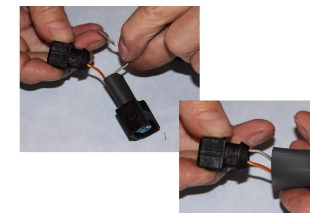
6. Twist wires together as shown below.
