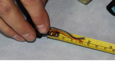
2. Cut each connector from the harness leaving 45mm of wire to allow the new connector to be fitted.
