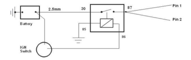
NOTE - 2.5mm Core wire must be attached directly onto battery +ve post.
