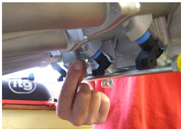
Adjusting the throttle stop screw
