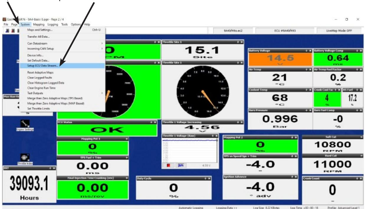
Please note there is an option for 'CAN Databstream' in the System dropdown, this is for older devices that have been set up in the past such as most AiM templates.
