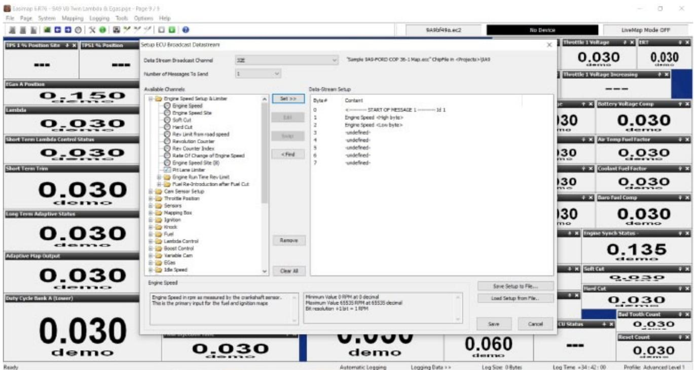
There are currently 2 channels set in the example below, engine speed and coolant temp. Both of these are being set up in 16 bit, RPM will always need to be 16 bit because it is 1 rpm per bit. Coolant temp is also being set in 16 bit, but this is quite often set up in 8 bit since it does not normally require accuracy greater than 1 degree centigrade.
