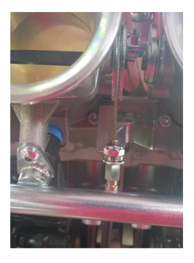
The SBD Inline adjuster can be placed anywhere in the cable run, select a position which allows access.
