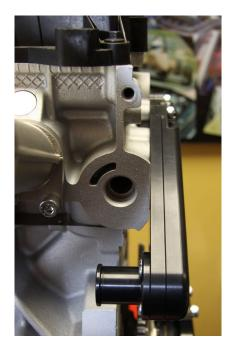
Bolt the water rail on to the cylinder head as shown below, ensuring the o-ring inside is in place
