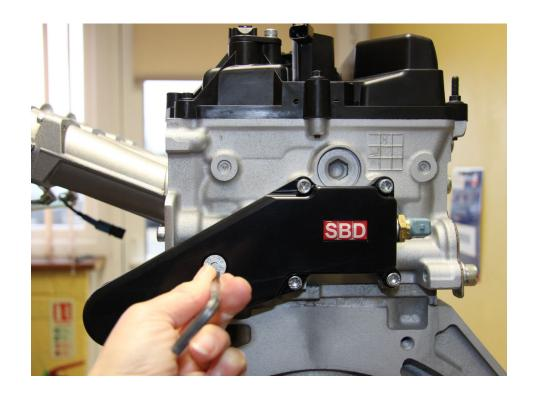
The bleed fitting can been fitted to either of the 2 holes on the top of the water rail.
