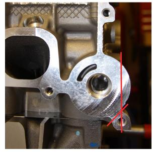
Using a hack saw, trim the back of the cylinder head as shown left and below to enable the WT-DURA-4K to fit flush to the edge
